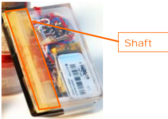
Figure 4. Images of a prototype M2E devices; the orange shaded rectangle in our belief represents a shaft for a sliding magnetic core.
